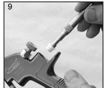
9. Fit New Front Seal to Service Tool.
