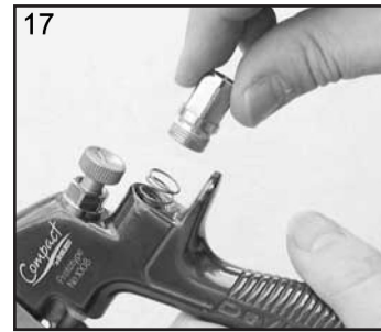
17. Replace Valve Spring and attach Housing (10).
