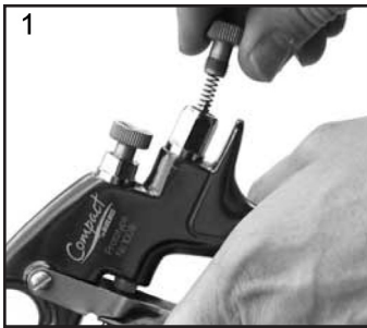
1. Remove Adjusting Knob (7), Spring (8), and Needle (9).
