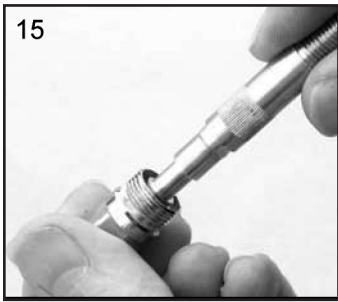
15. Fit Seal to Housing (10).
