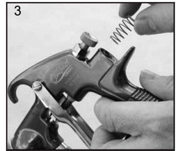
3. Remove Housing (10) and Air Valve Spring.
