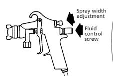
**Spray width adjustment:** Turn clockwise for round, counterclockwise for fan.
