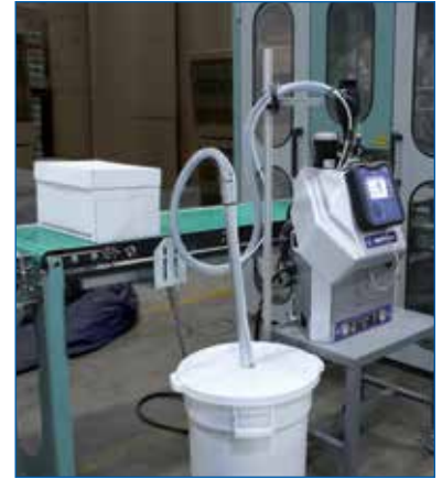
Since tank-free hot melt systems are compatible with a range of adhesives, packaging companies now have more material options.
