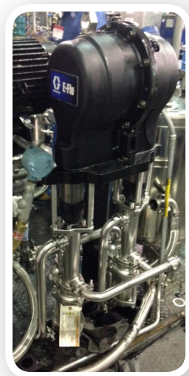
Legacy E-Flo Output up to 4000 cc/cycle
