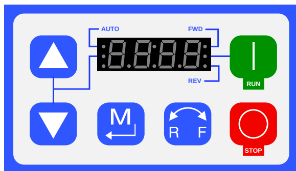
Figure 15 VFD Control Panel
