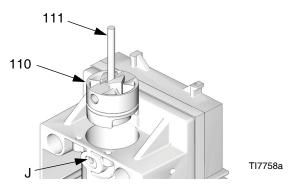
FIG. 10. Remove Piston Stops
