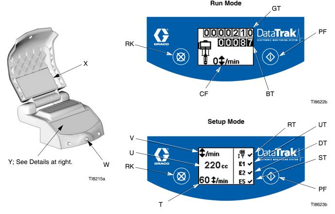
FIG. 3. DataTrak Controls and Indicators
