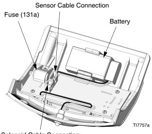
Solenoid Cable Connection FIG. 5. DataTrak Battery and Fuse Location
