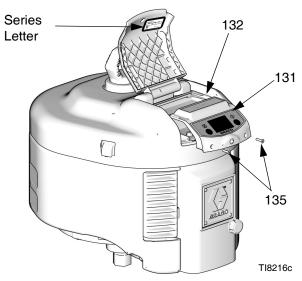
FIG. 4. Remove DataTrak Module
