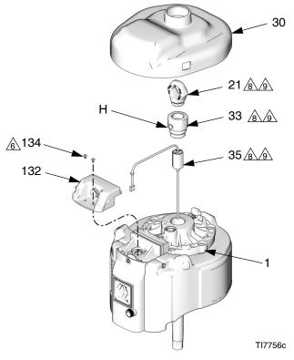
FIG. 16. Replace the Linear Sensor
